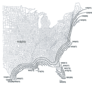
Figure 1.1 IBC Basic Wind Speeds: Basic Wind Speeds: Risk Category II. Source: ASCE 7-16
